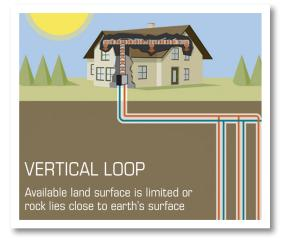
Vertical loops use drilling equipment to bore small-diameter holes from 50 to 200 feet deep. Piping is then fed down these holes creating a loop pattern. The individual loops are all joined together and tied to the indoor heat pump unit.
